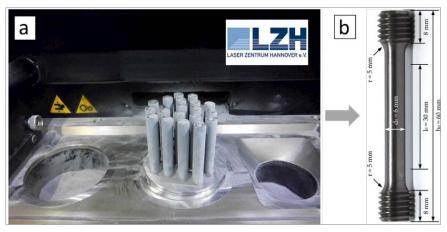
Figure 12. Tensile test set of Ti-42Nb PBF-LB built specimens fabricated by Laser Zentrum Hannover
